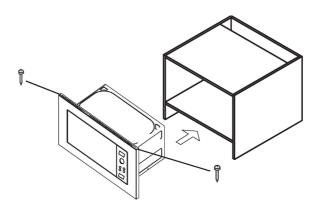
1. Put the microwave oven into the cabinet and keep the microwave oven in a horizontal direction and keep the edge distance of two side as same. Then fix the bolt (component 1) on the top of microwave oven and beat it into the cabinet.
