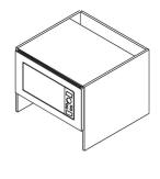
2. Open the microwave oven, fix the bolt (Component 3) and beat it into the cabinet, then install screw cover.
